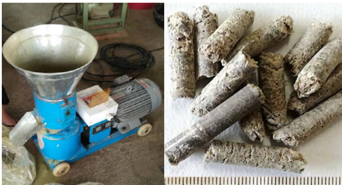
Fig. 1: A flat-die pelletizing machine and the PET/biomass pellets
