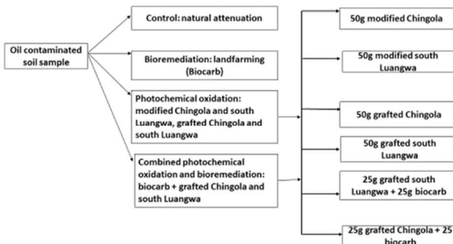
Fig. 3: Contaminated soil sample treatment setup (Effendi and Aminati, 2019)
