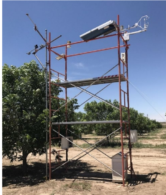
Fig. 1: Pecan nuts of 7-year-old trees and the sensors for eddy covariance measurements of the CO 2 net ecosystem exchange (NEE) and photosynthetically active radiation (PAR) above the trees' canopy
