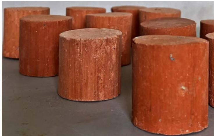
Fig. 1: Samples of fired test bricks
