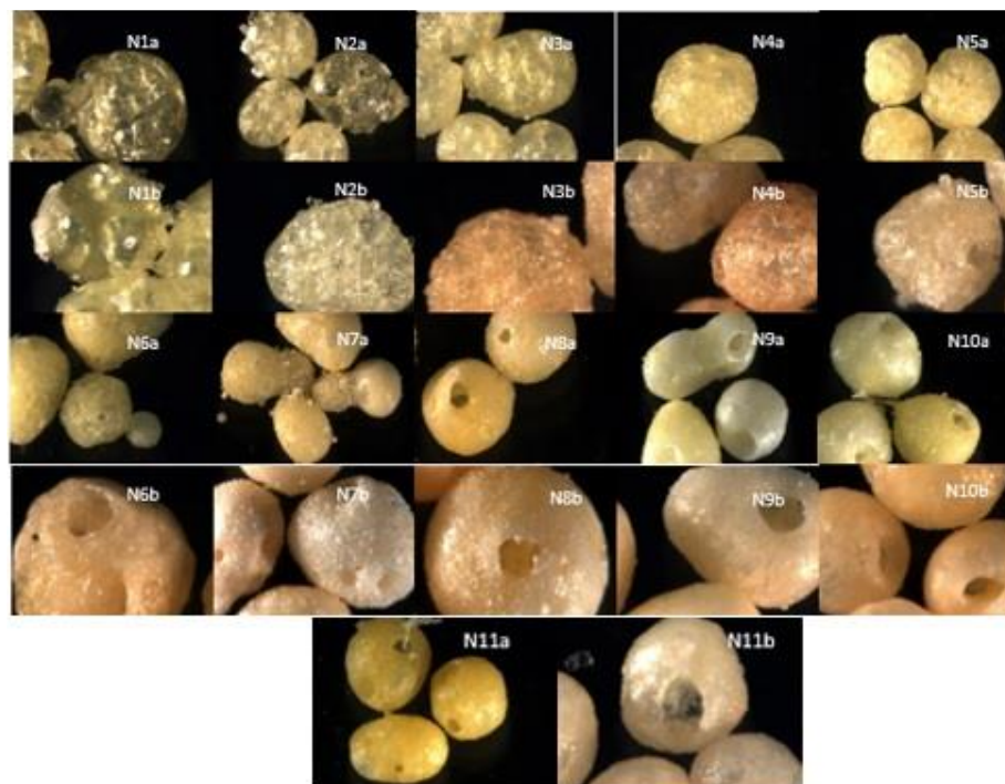
Fig. 3: Morphology of nifedipine microcapsule PLA:PCL (%w/w) (a) before dissolution 25x (b) after dissolution 50x
