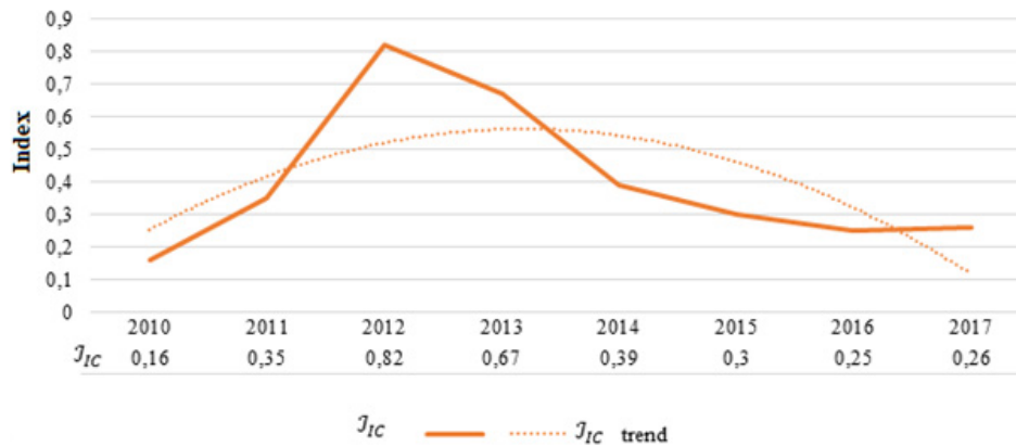
Fig. 1: Installed capacity index of NCRE technologies in Ukraine and Chile and graph of its dynamics 2010 vs 2017
