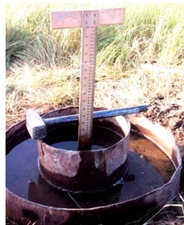
Fig. 3: Permeability determination by double ring method in the first layer of rainfed farming
