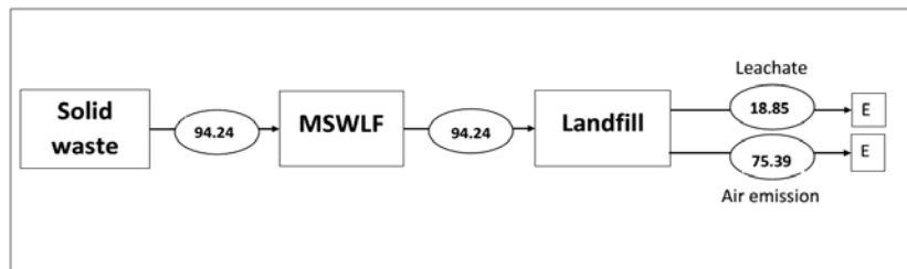
Fig. 6: Flow diagram of existing waste at MSWLF Troketon
