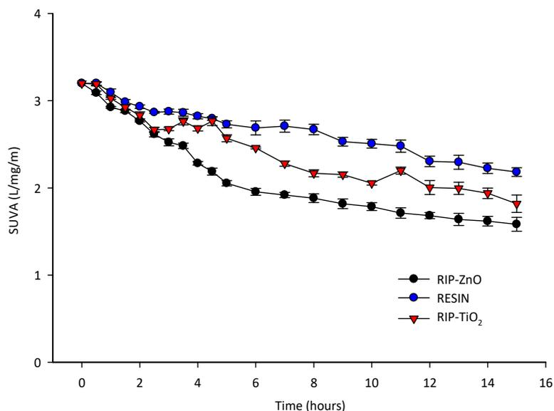
Fig. 3: The changing of SUVA value in tofu wastewater under various processes of resin, RIP-TiO<sub>2</sub>, and RIP-ZnO
