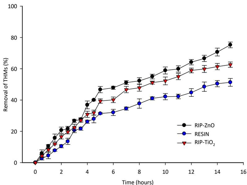
Fig. 4: The changing of THMs concentration in tofu wastewater under various processes of resin, RIP-TiO<sub>2</sub>, and RIP-ZnO
