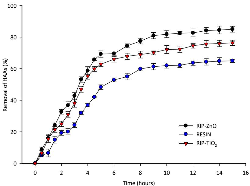
Fig. 5: The changing of HAAs concentration in tofu wastewater under various processes of resin, RIP-TiO<sub>2</sub>, and RIP-ZnO
