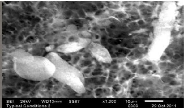
Fig. 13: SEM analysis of particles within depth of PVC filter
