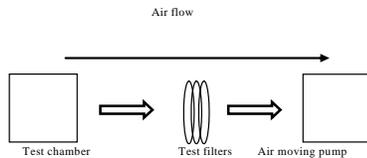
Fig. 1: Test chamber assembly set up
