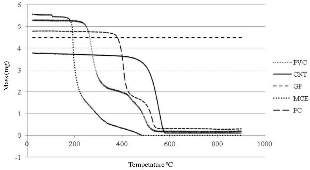
Fig. 5: CNT sample and test filters TGA traces
