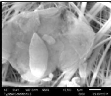
Fig. 3: CNT agglomerates on the face of a glass fiber filter
