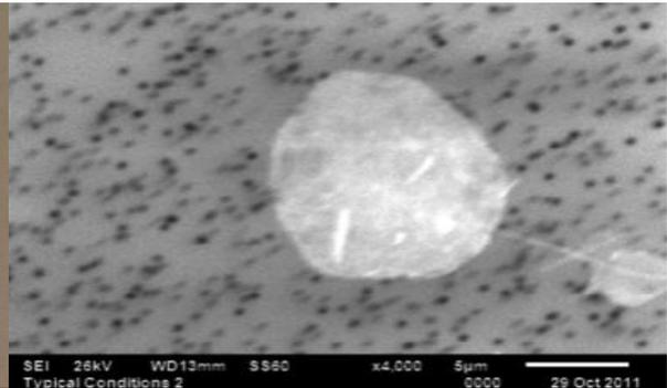
Fig. 11: SEM analysis of particles on the surface of PC filter
