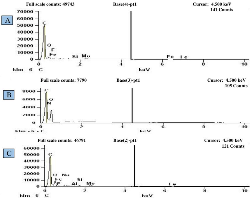
Fig. 15: Mixed cellulose ester filter spectra
