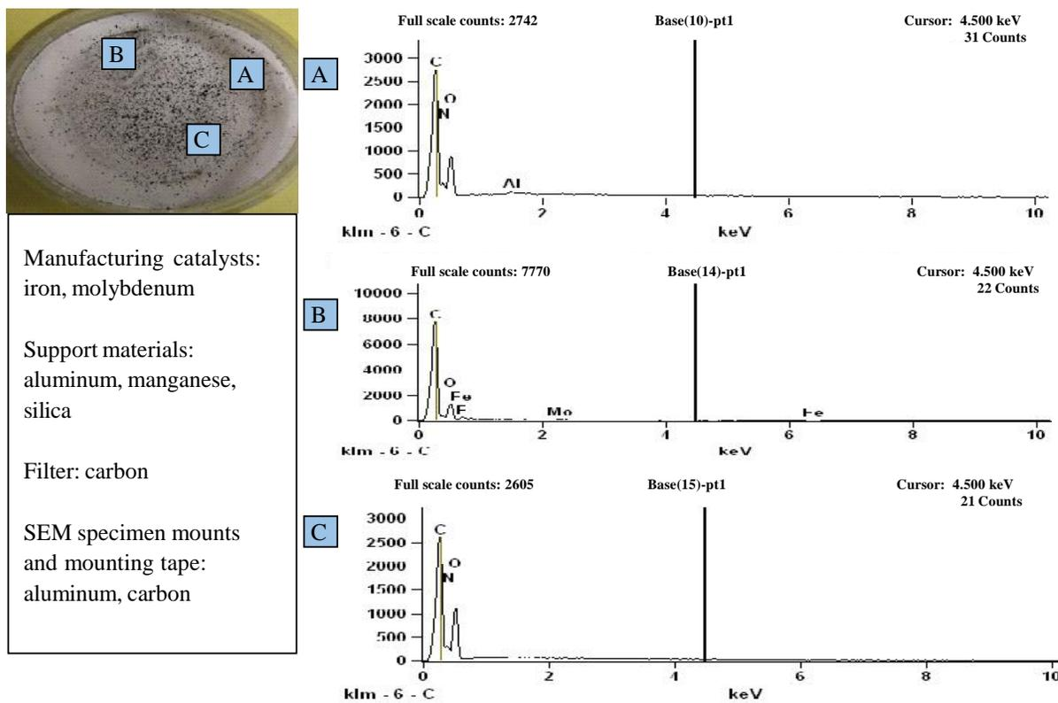
Fig. 17: Polyvinyl chloride filter spectra
