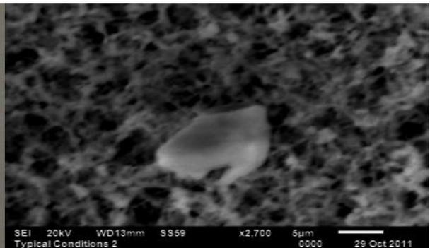
Fig. 9: SEM analysis of particles within depth of MCE filter
