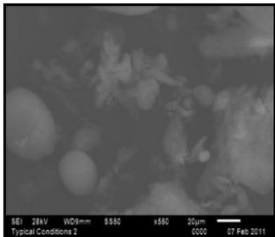
Fig. 2: CNT agglomerates on carbon adhesive tabs
