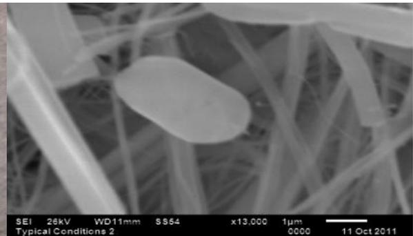
Fig.7: SEM analysis of particles within depth of GF filter
