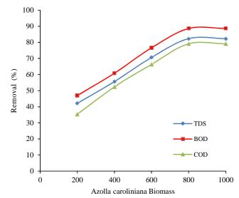
Fig. 3: Effect of Azolla caroliniana biomass on removal of TDS, BOD and COD from paper mill effluent
