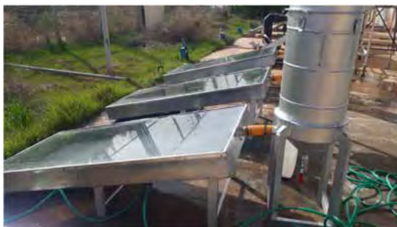
Fig. 5: Solar panels used for hot air and the disinfection unit
