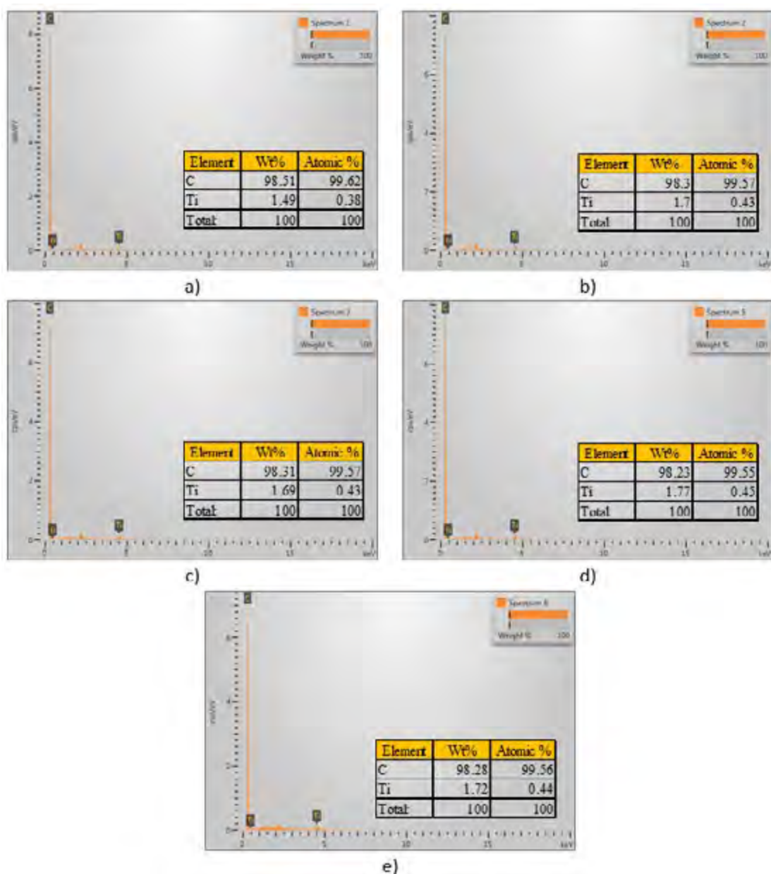
Fig. 5: EDX spectra of LDPE plastic biodegradation: a) Control (before biodegradation), b) IBP-1, c) IBP-2, d) IBP-3, and e) IBP-4 (after biodegradation)
