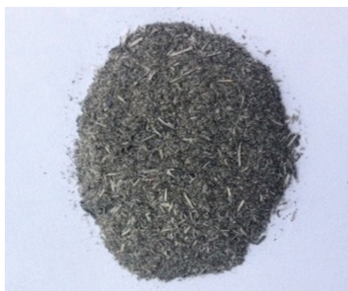
Fig. 4: Rice husk ash (500 °C for 4 h)
