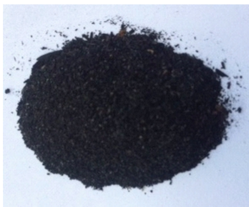
Fig. 2: Rice husk carbon (300 °C for 1 h)
