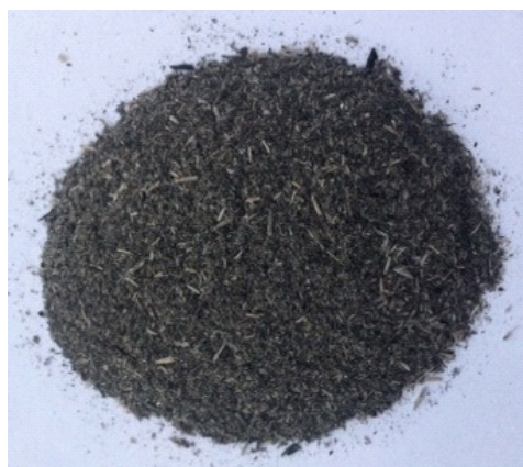
Fig. 3: Rice husk ash (400 °C for 2 h)
