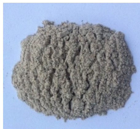
Fig. 5: Rice husk silica (650 °C for 6 h)
