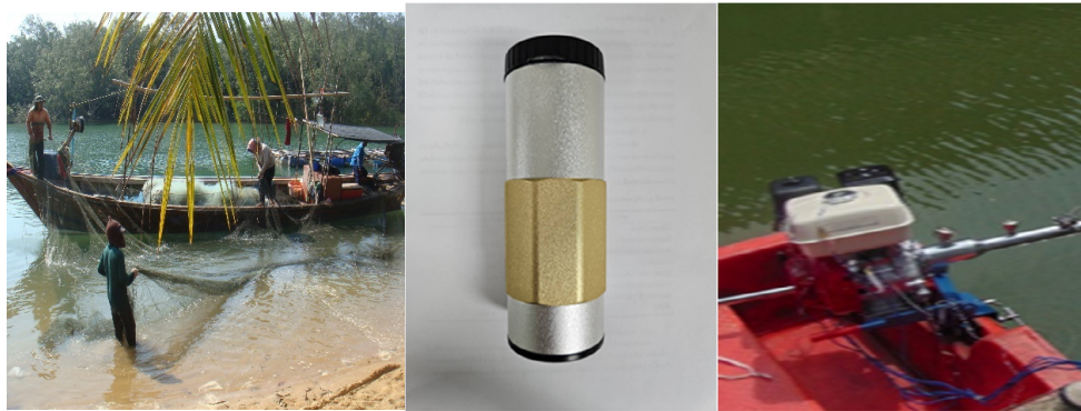
Fig. 3: silencer on the boat engine's exhaust pipe
